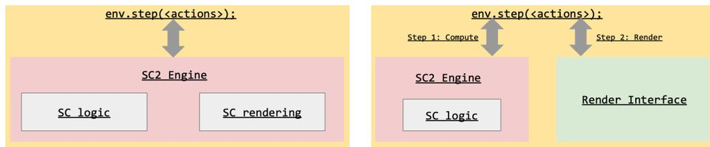
Figure 3.2: The figure on the left is a high-level architecture diagram showing the design of SMAC. The figure on the right shows our initial proposal for SMAC-lite.
